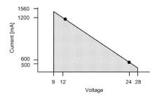
Maximum HOLD CURRENT should fall below the curve in the shaded region in order to achieve optimum coil life. The curve represents the temperature stabilized power of 14 watts.
