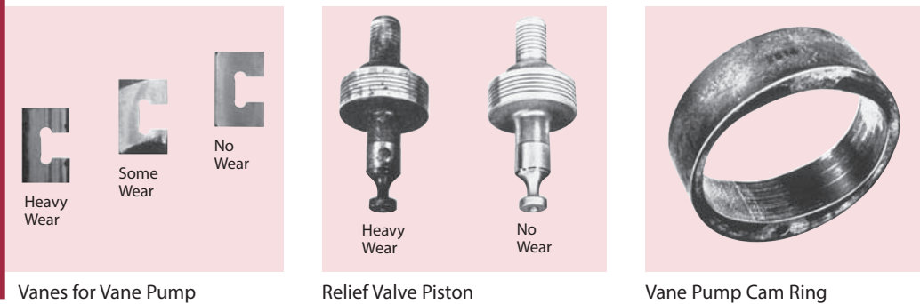
Figure 1. Typical Examples of Wear Due to Contamination
