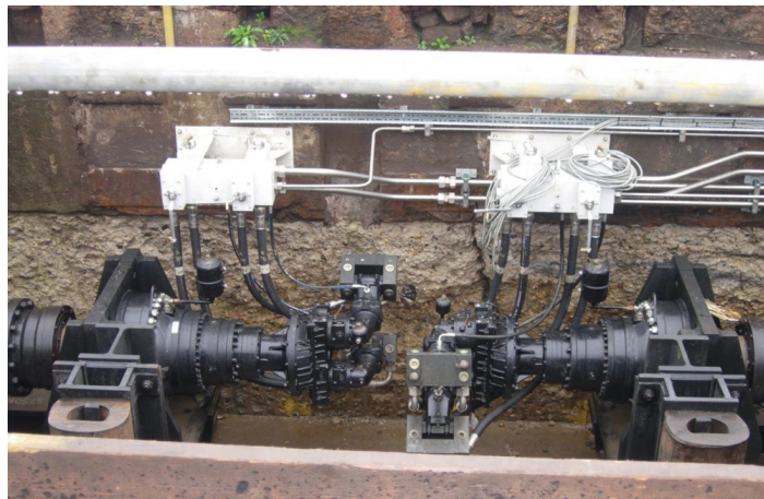
Dual Shuttle Drive Mechanism Photograph courtesy of Ipswich Hydraulics
