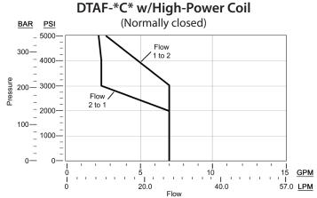
Note: The DTAF-\*H\* normally open valve cannot use the low-power coil.
