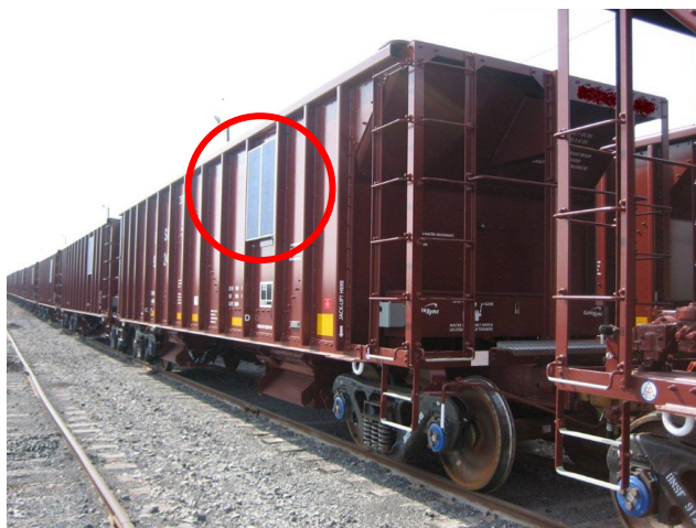
Ballast car mounted solar cell panel for recharging 24VDC battery pack
