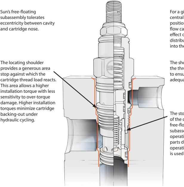
For a given thread size, the central location of the thread position results in maximum flow capacity, minimizes the effect of eccentricity, and distributes thread loads deep into the manifold.
