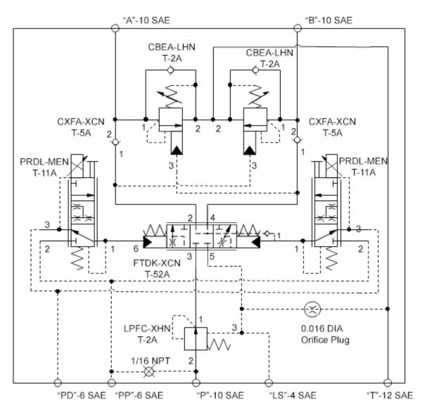
Figure 24 - Complete Proportional Cushion-Lock Manifold with Load Sensing
