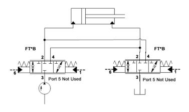
Figure 18 - Two 3/3-Way FT\*B valves create a 3/4-Way, closed-center function.
