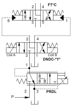
Figure 10 Two Electrical Pilot Control Options
