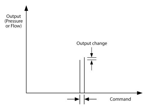
Smallest change in command which produces a measurable change in output.
