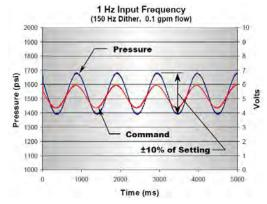
With low frequency, input command and output pressure remain in phase. Output pressure rises fully.
