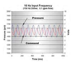
With high frequency, output pressure lags input command. Output pressure does not rise fully.
