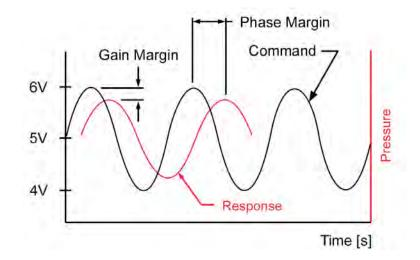
• The key point for hydraulic valves is -3 dB, which means that the response of the valve is 71% of the commanded value. Phase margin is a measure of how well the valve is tracking in time the commanded value. Phase margin is measured in degrees and can either be leading the command value (very unlikely in hydraulic valves) or lagging (more common in hydraulic valves). The key point of phase margin is -90°, which means the valve response is lagging the command by 90°.
