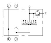
The oil passed through the hot oil shuttle valve goes across a lowpressure relief valve set at a slightly lower pressure than the charge pump. This oil is taken through an offline filtration and cooling unit before being returned to the oil reservoir. Often this oil is also passed through the casing drain of the transmission motor to help keep the motor cool.
