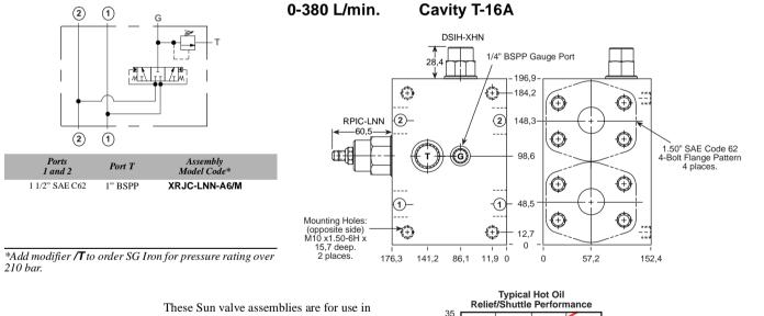
bleeding hot oil from the low pressure side of a hydrostatic transmission circuit. The hot oil can be cooled, filtered, or used as a source of oil for flushing other pump and motor cases. The hot oil is removed from the loop when the Sun RPIC cartridge is set below the hydrostatic charge pressure relief valve.
