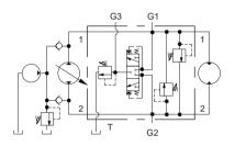
The hot oil shuttle valve senses pressure from the high-pressure side and opens to bleed off oil from the return low-pressure side of the circuit. A low-pressure charge pump into the inlet of the transmission pump makes up this oil.
