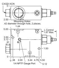
\*Add modifier /S to order Ductile Iron for pressure rating over 3000 psi.
