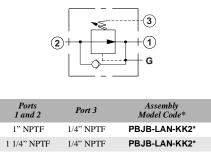
\*Add modifier /S to order Ductile Iron for pressure rating over 3000 psi.
