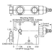
\*Add modifier **/S** to order Ductile Iron for pressure rating over 3000 psi.
