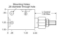
FULLY ADJUSTABLE NEEDLE WITH REVERSE FREE FLOW CHECK
