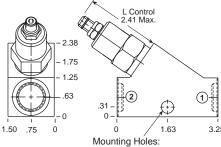
Mounting Holes: .42 diameter through hole.
